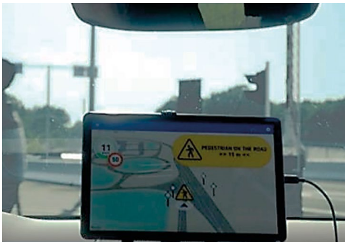
Figure 5: HMI developed for positions view and alert message
