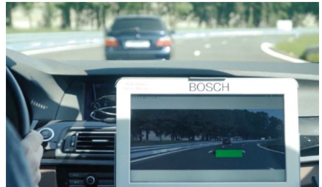
Figure 3: See-through HMI inside the rear vehicle
