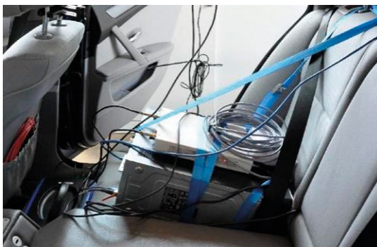
Figure 4: V2V hardware integrated into vehicle
