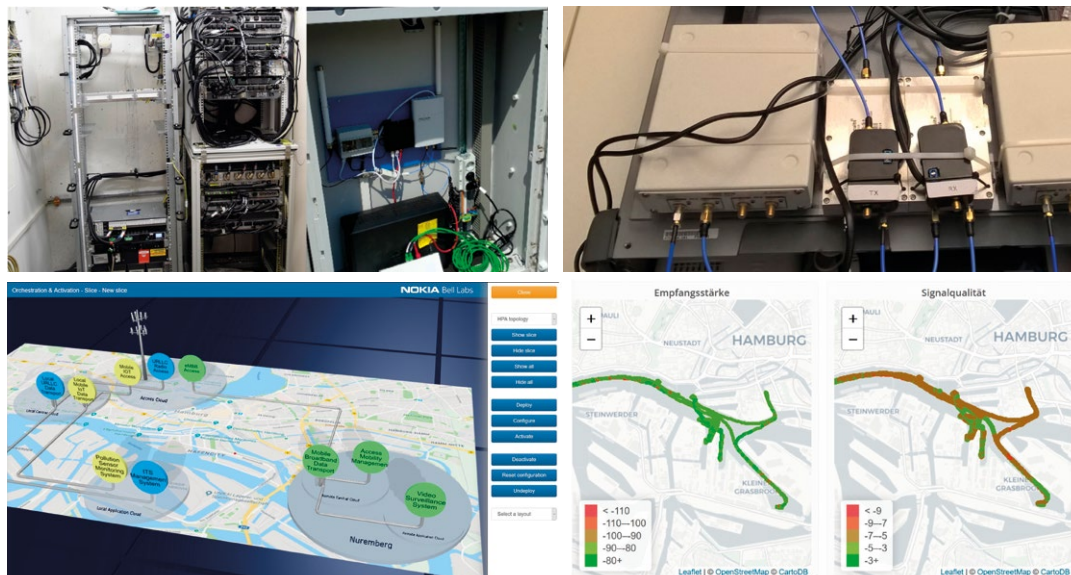
Figure 2: Base station at Hamburg TV tower (upper left), device installation for traffic light (upper middle), multi-connectivity device as installed on barges (upper right), visualization tool (bottom left), excerpt of the KPI panel (bottom right)
