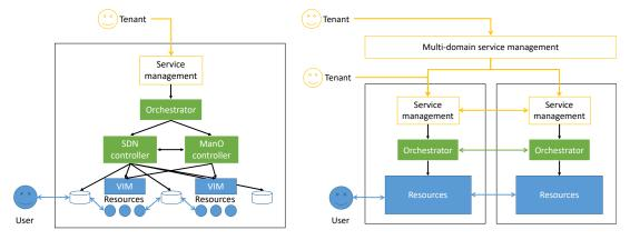
Figure 5-1 Meta-architecture for single-domain case (left) and multi-domain case (right)
