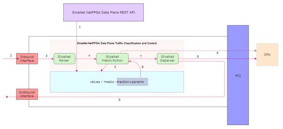
Figure 4-24 Programmable data plane prototype (HW-based)
