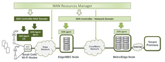
Figure 2-7: SDN architecture for data plane programmability [2-14]
