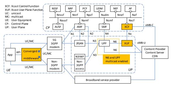
Figure 4-1: System architecture enhanced for multicast and broadcast.
