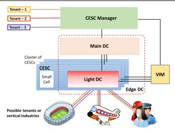
Figure 2-8: Proposed functional architecture [2-16]; DC stands for Data Centre
