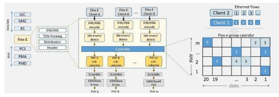
Figure 4-8: Flex-E layer between Ethernet MAC and PCS. Additional FlexE Shim distribute/aggregate sub-layer in PCS/PMD.
