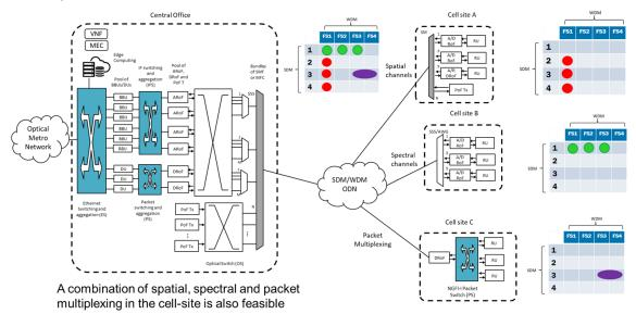
Figure 4-13 SDM-enabled infrastructure architecture
