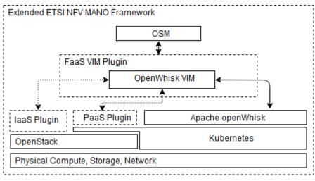
Figure 2-12: Extending ETSI MANO Reference Architecture with FaaS
