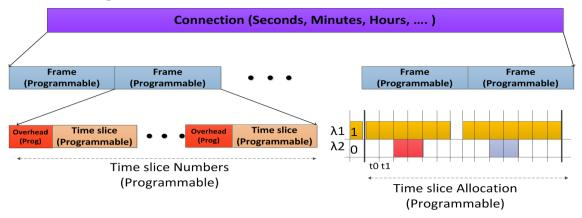
Figure 4-5: Structure of connection, frame and burst.
