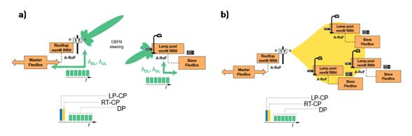
Figure 4-22 (a) Data Plane pencil beams (b) The Control Plane wide beam antennas
