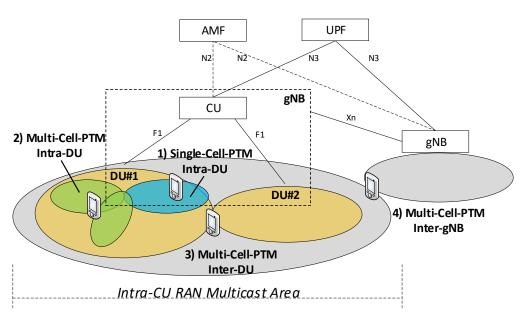
Figure 3-9: Deployments of the RAN Multicast Area, in function of single gNB
