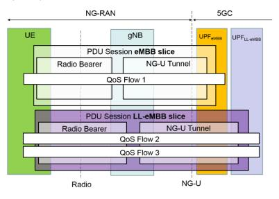
Figure 3-4: Network Slice support in the 5GS.
