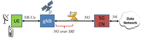
Figure 3-13: Regenerative on-board non-terrestrial platform
