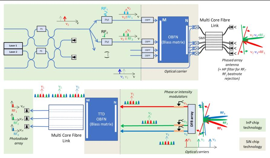
Figure 3-23: Coherent OBFN-based downlink transmitter – receiver
