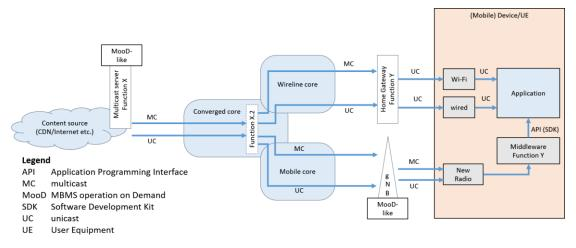
Figure 2-11: Framework for efficient content delivery over 5G networks [2-27].
