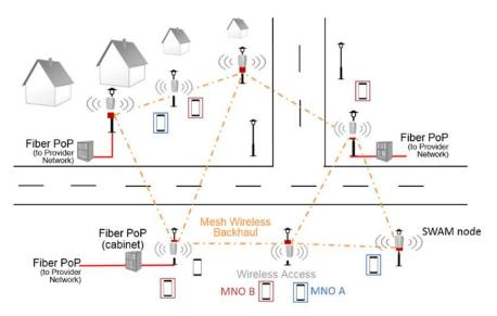
Figure 4-16: Deployment scenario for the joint access-backhaul function.
