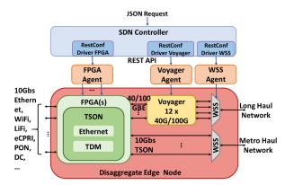
Figure 4-12 Disaggregated edge node architecture
