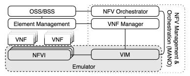
Figure 6-3: Scope of the emulation platform in the simplified ETSI NFV reference architecture
