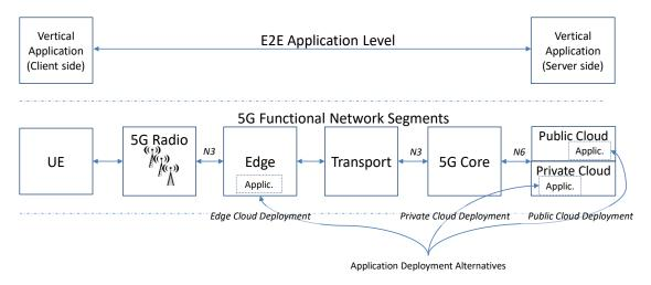
Figure 6-1 Functional Network Segments of a 5G System
