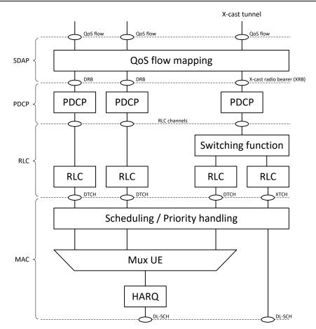
Figure 3-11: L2 architecture and bearer selection in Cloud-RAN
