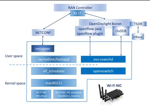
Figure 3-5: Wi-Fi virtualization and slicing
