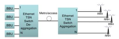
Figure 4-9: Ethernet TSN network for aggregation, transport and de-aggregation in FH.
