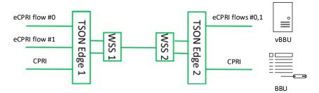
Figure 4-7: Multiplexing of eCPRI and CPRI over TSON.
