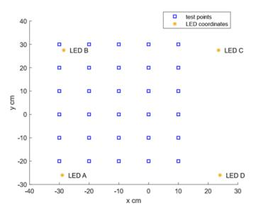
Figure 5-68 The distribution of the 30 test points and the coordinates of the four LEDs
