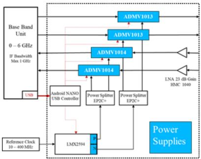
Figure 4-34 Internal architecture for the compact mmWave transceiver module
