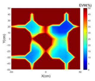
Figure 5-63 4 VLC LED TXs EVM test Rx at ground level pointing vertically up LED A and illumination LEDs off – top Right, B – bottom right, C – bottom left, D – top left
