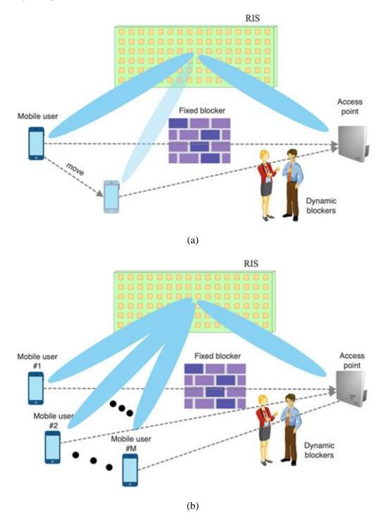
Figure 4-38 (a) RIS-assisted beamforming, and (b) RIS-assisted broadcasting
