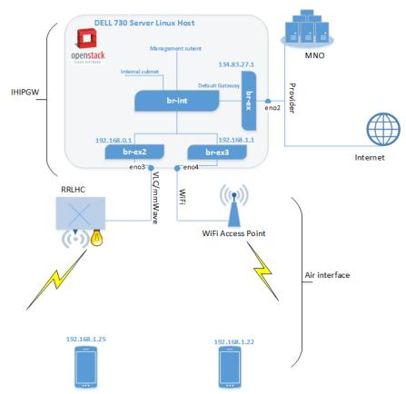
Figure 4-42 Illustration of the network architecture including MEC cloud
