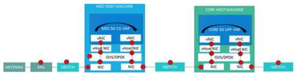
Figure 4-53 Hybrid data plane network slicing
