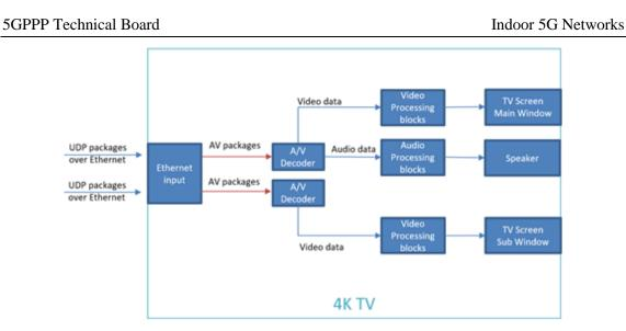
Figure 6-73 Basic diagram of Android based 4K TV application
