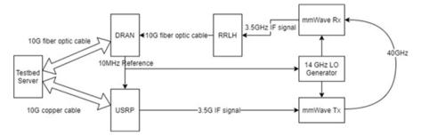
Figure 5-65 Testbed system setup for mmWave uplink measurement
