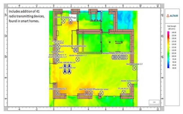
Figure 5-62 Measurement of EM radiation in integer house upper Ground floor – addition of multiple sources of radiation
