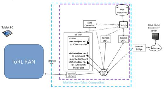
Figure 4-47 Integrated security framework in MEC
