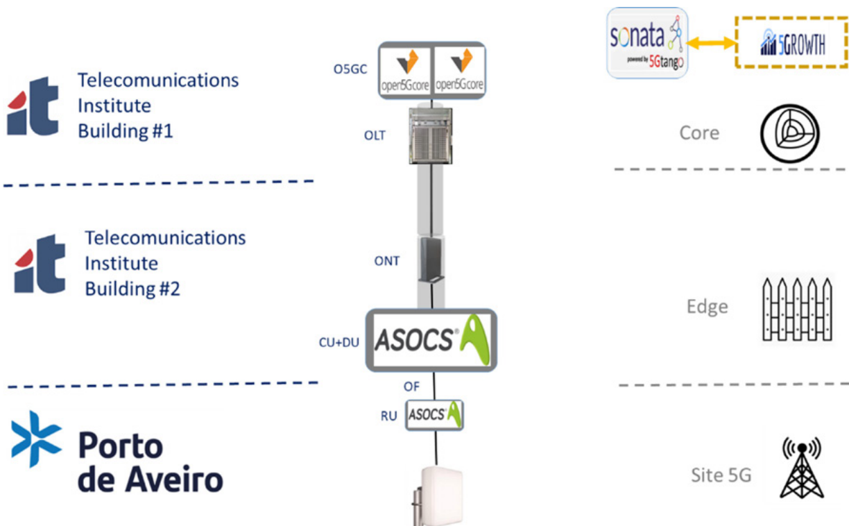
Figure 2: Transportation pilot - 5G infrastructure
